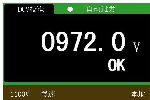
Figure 8-2 DC voltage calibration is completed
