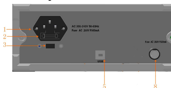
Figure 3-4 ET1240 Rear panel diagram (standard part only)
