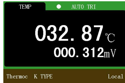
Figure 5- 16 Thermocouple temperature measurement
